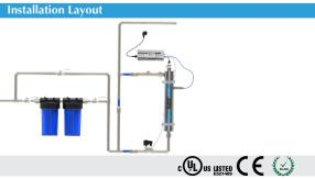
Ultraviolet light treatment is a widely recognized and proven method of disinfection of water, does not add anything to the water, nor does it generate harmful byproducts. It adds only energy in the form of ultraviolet radiation. It is fast, efficient, effective, economical and environmentally-friendly.
